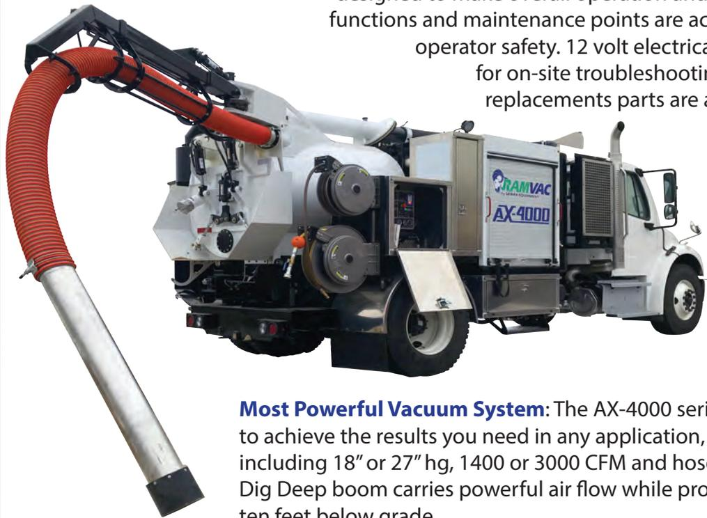
**Does It All:** This one machine provides the ability to pothole using a 4" port, as well as conduct major excavating utilizing a 6" port. The AX-4000 series offers standard payload capacities from 5,000 to 12,000 lbs. while its hydraulic rear door allows operators to dump spoils quickly and easily.
