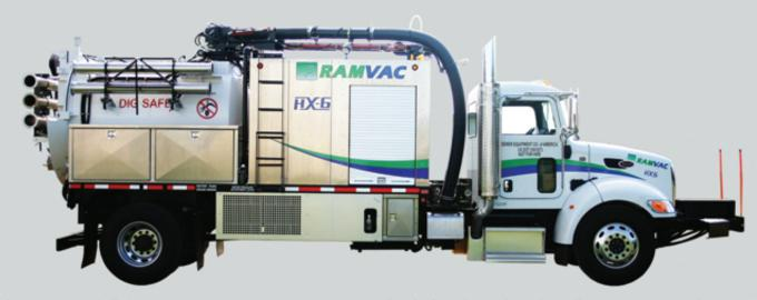
The RamVac 6" Vacuum-Excavators are purpose built for the job. The 6" system mated to a 3000 CFM/18"HG Positive Displacement Blower gives you 180+ MPH air flow to move material as fast as you can cut it. The 6" Truck is available in highly maneuverable 3yd and 6yd configurations or in 9yd and 12yd to accommodate continuous digging without the need to dump.
