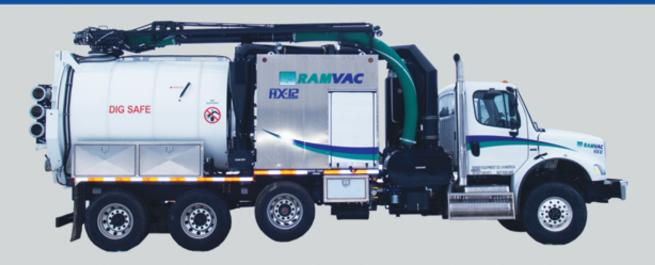
The RamVac 8" Hydro-Excavators delivers not only class leading Hydro-Excavation capabilities but give you the ability to bulk load material as well. The 8" systems 5500 CFM/27"HG Positive Displacement Blower has the unique ability to be activated from the system control panel so you don't have to go to the cab to activate your blower. The RamVac HX in 8" is also the only Excavator in its class to offer the Temperature Controlled Environmental Chamber to prevent our water system from freezing.
